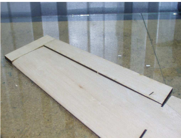
Figure 3.15: Elevon lined up before shaping
