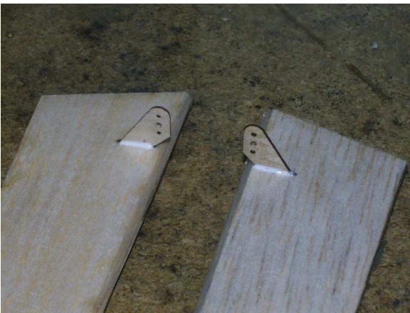
Figure 3.19: Elevon control horns installed
