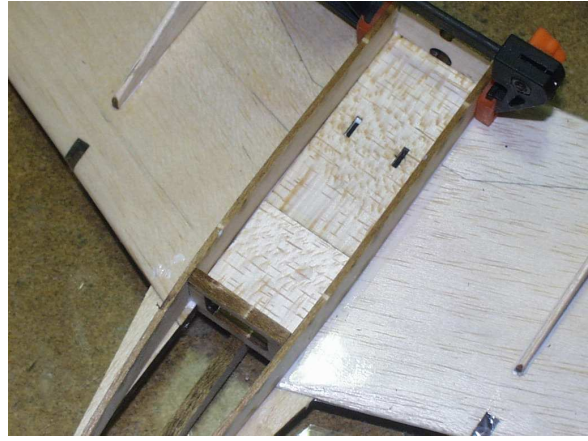
Figure 4.11: Both reinforcement plates installed
