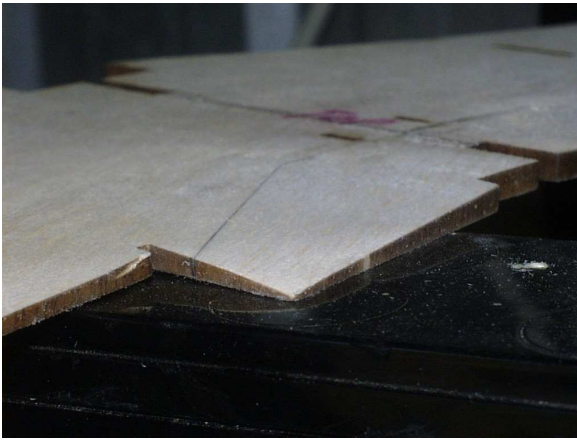
Figure 3.10: Trailing edge detail at wing center
