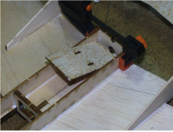
Figure 4.10: Inserting reinforcement plate
