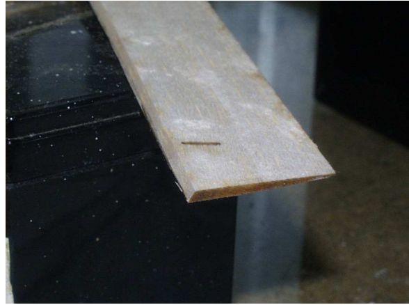
Figure 3.18: Elevon after beveling
