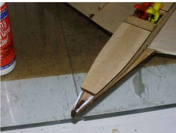
Figure 4.23: Gluing the front fixed hatch
