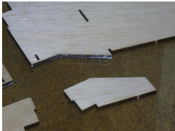
Figure 3.2: Notice the limited amount of glue.
