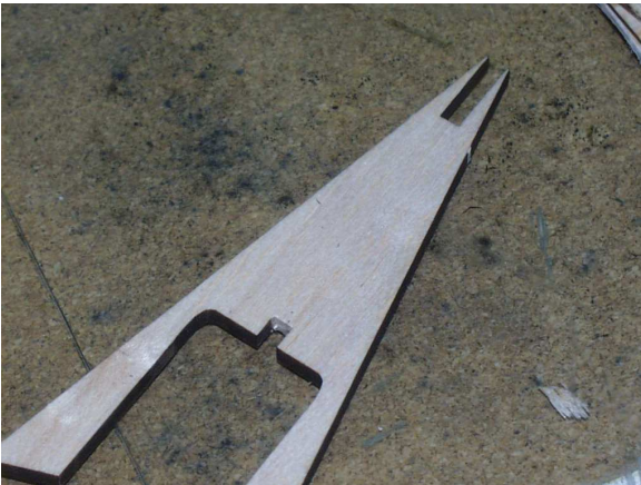
Figure 4.1: Small recess cut away in spike
