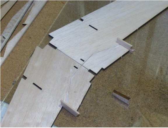
Figure 3.3: Joining of the wing halves.
