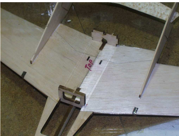
Figure 4.8: F1 and F2 installed
