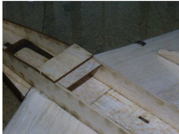
Figure 4.19: Rear tongue installed for alignment
