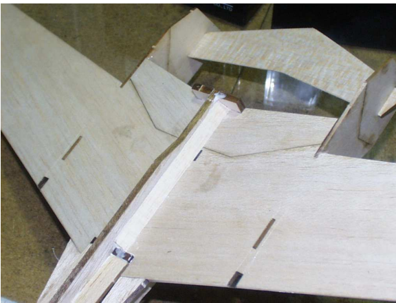
Figure 4.16: Installing the triangle stock
