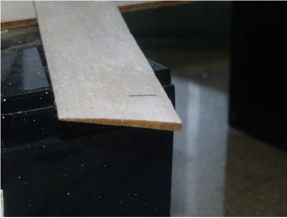
Figure 3.17: Elevon before beveling
