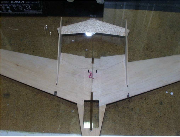
Figure 4.6: Check booms are parallel
