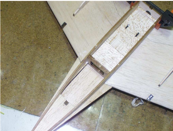
Figure 4.12: Battery bay plate installed
