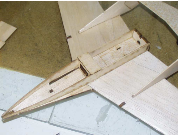
Figure 4.18: Rear fixed deck installed
