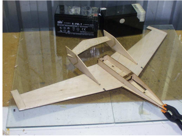
Figure 4.15: F1 doubler installed
